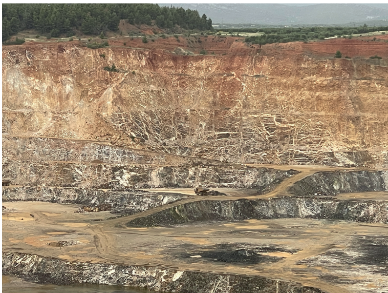
Fig. 3 Ore veins: The cryptocrystalline magnesite vein stockwork, hosted by dunite, is easily observed at one of the working pits at Grecian Magnesite's Yerakini mine, Halkidiki, Greece, site of the MagForum 2024 Field Trip. About 500 000 t/a of dunite and magnesite is co-extracted, feeding three rotary and one shaft kiln with a total combined calcination capacity of about 180 000 t/a
