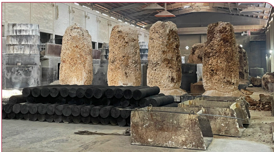
Fused magnesia ingots cooling before being broken and sorted into grades, with new graphite electrodes in the foreground for use in the EAFs, at Haicheng Magnesite Group's plant in Haicheng, China
