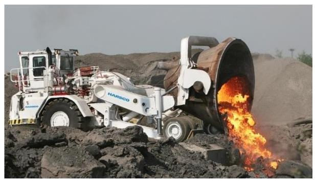
Recovery of steel slag by Harsco Metals & Minerals for re-use in markets such as construction, fertiliser, and filter media. Courtesy Harsco Metals & Minerals.
