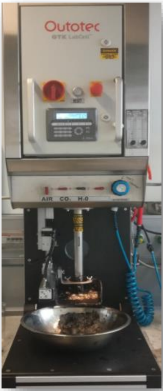
A 2L Outotec cell (GTK labCell)
