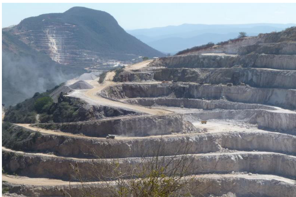
Forthcoming merger: Magnesita's vast Pedra Preta magnesite mine, near Brumado, Bahia, Brazil, which provides more than 1 million mt/year feedstock for dead burned and caustic calcined magnesia production, could be joining RHI's equally impressive magnesite resources in Austria. (Ibar Nordeste's magnesite mine is in the background, soon to be exporting its DBM production). Photo courtesy of IMFORMED
