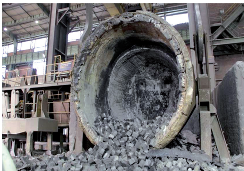
Fig. 3 Refractory wreck-out: a steel ladle disgorges its spent refractory brick lining – once a waste product bound for expensive landfill sites, now a keenly sought after secondary raw material. (Courtesy Sidenor9
